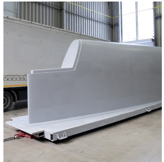
Modular Plug made by METYX Composites
