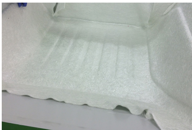
METYSORE laying into the mould
