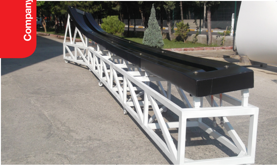
Epoxy heated mould for wind blades
