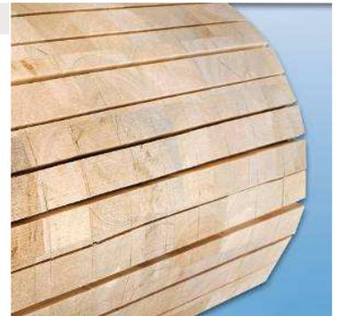
BALTEK® SB is a core material produced from select kiln-dried balsa wood in the 'end-grain' configuration. It has extremely high strength and stiffness to weight ratios, and achieves an excellent bond with all types of resins and adhesives.
